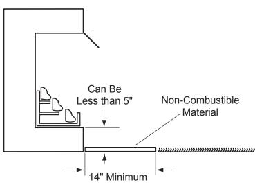
Figure 8 - Minimum Clearance above Combustible Flooring with Non-Combustible Material Installed at Base of Fireplace
